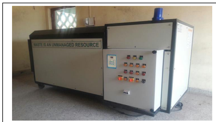
Figure 1: Typical OWC (Organic Waste Composting) Plant
